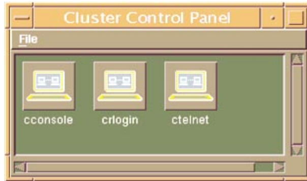
FIGURE 2-6 Cluster Control Panel Window
